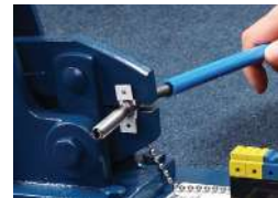
3. CRIMP ON REPLACEMENT COUPLING
