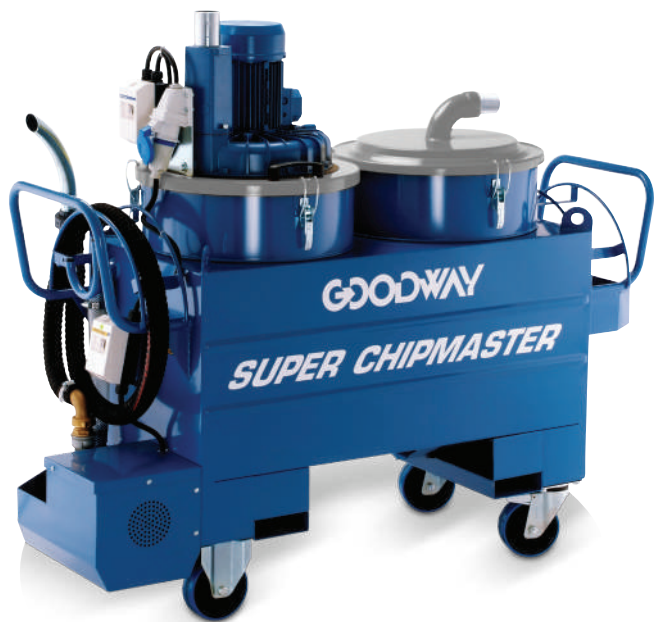
DV-CM4: Chip/Coolant Recovery Vacuum, including 22 gallon metal chip basket, nylon and polypropylene filters, 66 gallon liquid collection tank, handles, casters, transfer pump, and dump valve ....
